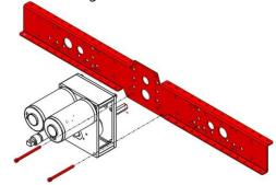
**Step 4**: Secure the #10-32 screws with #10-32 Nylock Nuts (am-1047) as shown. Install one 500Hex x 0.25" Spacer (am-3948-250) against the hex bearing on the output shaft of the Sonic Shifter.
