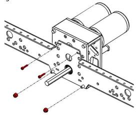
**Step 2**: Insert the two 1/4-20 x 3.00 SHCS into the side of the Sonic Shifter with the motors, then insert the hex shaft through the large bearing hole. Insert the 1/4 screws the into the two 1/4" diameter holes on the AM14U4 Inside Plate on the same side as the bottom flange.
