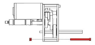
**Step 3:** Flip the inside plate over, and install two #10-32 x 0.75" SHCS through the inside plate into the Sonic Shifter. Install the two 1/4-20 Nylock Nuts onto the 1/4-20 Screws and tighten.
